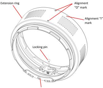
Locking tab for use with earlier version "pin locking" extension rings
