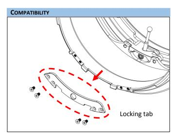
This extension ring is backwards compatible with other N120 extension rings. A user installable locking tab is pre-installed for this purpose.
